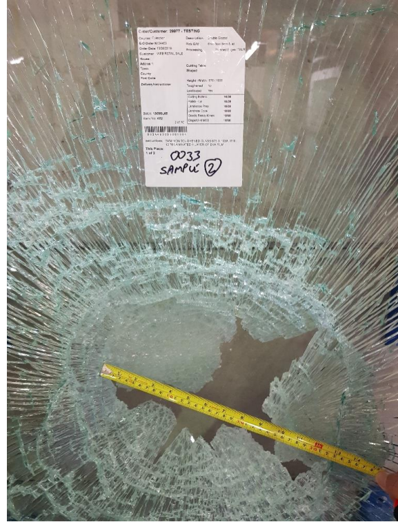
Sample 2 (broke unsafely)
